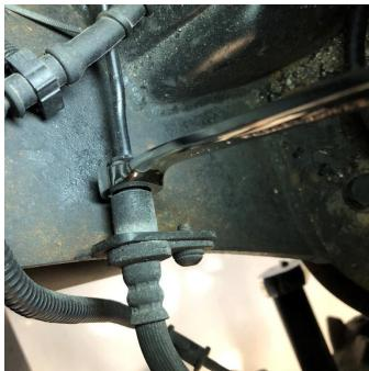
This installation refers to the passenger side. All steps are to be repeated on the driver side. Start by removing the factory brake line from the ABS wire and frame.
