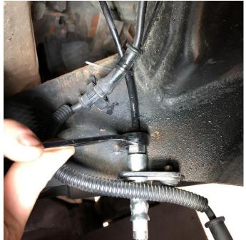
The Stainless Hoses can then be installed onto the caliper and factory hardline at the frame.
