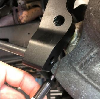
Once the rotor is removed, the backing plate will need to be marked and trimmed to allow clearance for the radial bracket.
