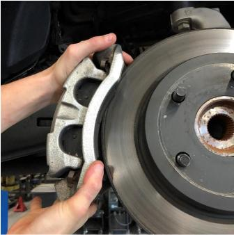
Remove the bolts connecting the caliper brackets to the spindle. The caliper and brackets can then be removed.
