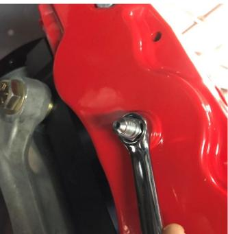
These Wilwood calipers utilize a 1/8 NPT fitting. **Do not thread any OEM tube-nuts into the caliper directly without adapting to 1/8 NPT.** This brake kit is available with an optional hose kit, which can also be purchased separately here:
