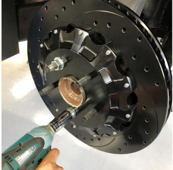
Arrange the rotor and hat in the position shown ensuring the arrow noting rotation direction is correct for its position on the vehicle. Start the first few threads of all 12 of the 5/16-18 x .875 bolts. Using an alternating sequence, apply red Loctite® 271 to the threads, and torque to **25 ft-lbs**. The rotor can be installed on the hub at this time using two lug nuts to hold the hat flat against the hub.
