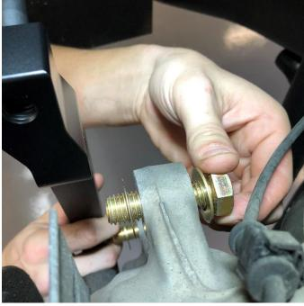
Once the backing plate is trimmed, the radial brackets can temporarily be installed at this time using the supplied 9/16 bolts and washers, along with two .563x1.125x.035 shim washers between the spindle and radial bracket.
