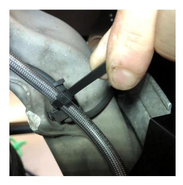
Using a small zip tie, attach the hose to the ABS wire to prevent any interference with surrounding parts.
